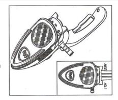
**Caution:** Always disconnect the iron before adjusting the dual voltage switch to the correct voltage setting.
